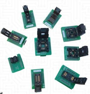
The universal pin driver on GSAS IUP-UXP enables you to support all 44-pin PLCC / QFP / PSOP / TQFP chips such as EPLD, EPROM, Flash, and Microcontrollers. For example one 44 pin PLCC adapter supports all 44 pin PLCC devices, which eliminates the need to buy multiple adapters.
