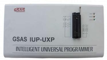
GSAS IUP-UXP is an advanced version of our earlier model GSAS IUP-XP, which works through a PC's parallel port & USB port. It features a 48pin universal pin driver and an expandable TTL pin driver. It supports over 7000 devices including PAL, GAL, CEPAL, EPLD, PEEL, MAX, MACH, PLSI, EPROM, MPU/MCU etc. GSASIUP-UXP works in various operating systems, Windows, 9x/NT/2000 and XP.
