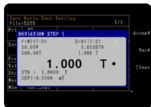
Inductive method/voltage method for measuring turns ratio
