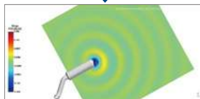
Acoustic analysis using fluid analysis results as a sound source
